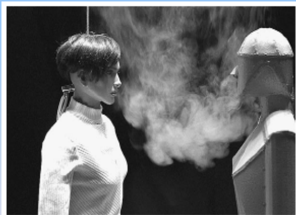
Figure 2 Smoke visualization of exhalation flow from nose of the right mannequin penetrating into the breathing zone of the left mannequin, which are 0.4 m apart. 94 reproduced from Figure 12 in Reference 94 with the kind permission of Blackwell Publishing.
